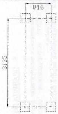
Scheme of the post placement with foundations
